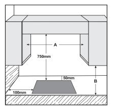
NOTE: if distance "A" between the kitchen cabinets is between 600 mm and 750 mm, height "B" must be at least 530 mm. If distance "A" between the kitchen cabinets is greater than the width of the hob, height "B" must be at least 400 mm. If a hood is installed above the hob, refer to the assembly instructions for the hood to see the necessary distance.
