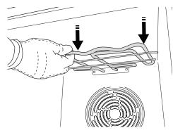
To return the heating element to its position, lift it up, pull it slightly towards you and make sure that the tab support is in its proper seating.
